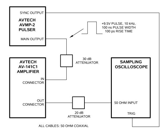
The recommended test set-up is shown above.
