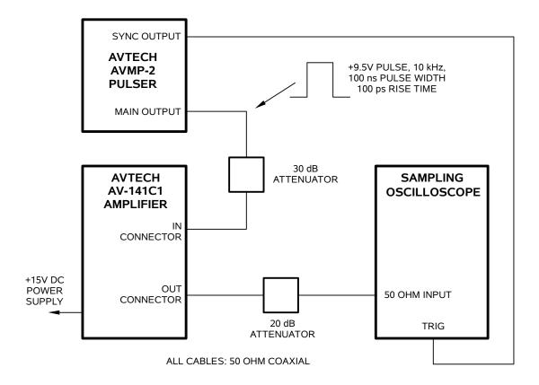
The recommended test set-up is shown above.
