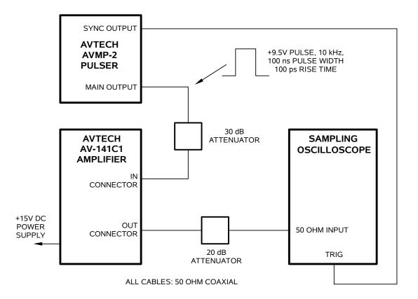
The recommended test set-up is shown above.
