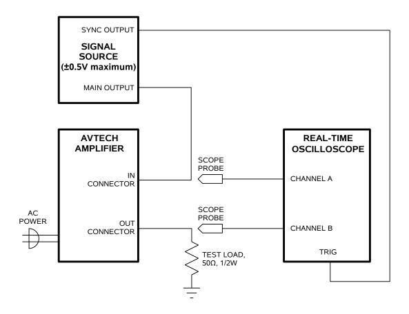
The recommended test set-up is shown above. The Avtech AV-1030-C pulse generator is a suitable signal source.
