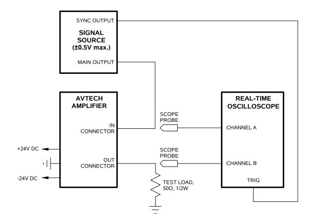
The recommended test set-up is shown above. The Avtech AV-1030-C pulse generator is a suitable signal source.
