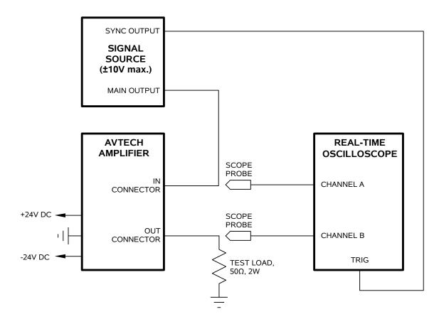
The recommended test set-up is shown above. The Avtech AV-1000-C pulse generator is a suitable signal source.
