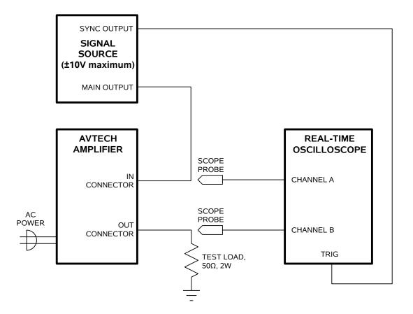
The recommended test set-up is shown above. The Avtech AV-1000-C pulse generator is a suitable signal source.
