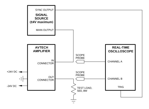
The recommended test set-up is shown above.
