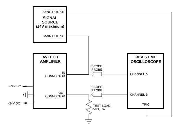
The recommended test set-up is shown above.
