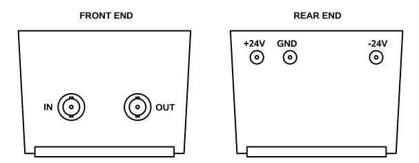
The input and output BNC connectors are located on the front end of the module, as shown above. The +24V, -24V, and GND input solder terminals are located on the opposite end.
