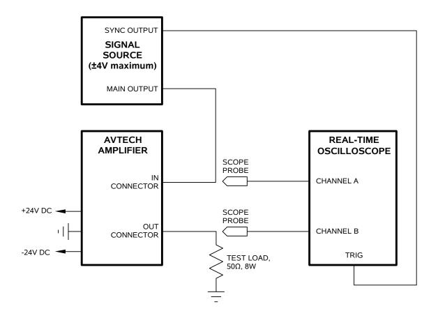
The recommended test set-up is shown above.
