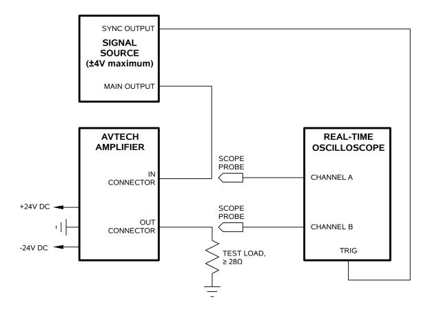
The recommended test set-up is shown above.
