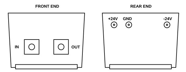
The input and output SMA connectors are located on the front end of the module, as shown above. The +24V, -24V, and GND input solder terminals are located on the opposite end.
