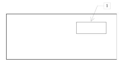
1. AC POWER INPUT. A three-pronged recessed male connector is provided on the back panel for AC power connection to the instrument. Also contained in this assembly is a slow-blow fuse and a removable card that can be removed and repositioned to switch between 120V AC in and 240V AC in.
