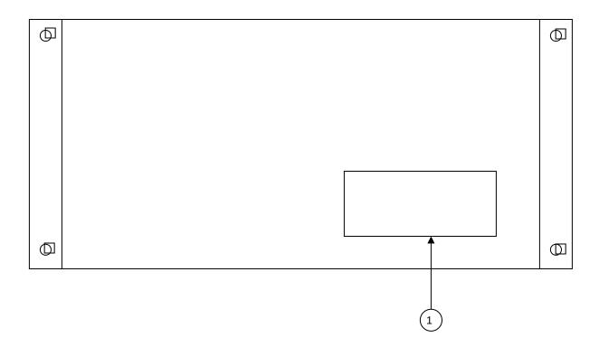
1. <u>AC POWER INPUT</u>. A three-pronged recessed male connector is provided on the back panel for AC power connection to the instrument. Also contained in this assembly is a 0.5A slow blow fuse and a removable card that can be removed and repositioned to switch between 120V AC in and 240V AC in.
