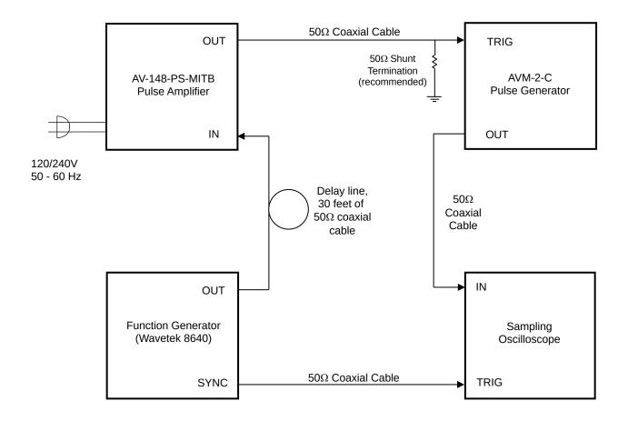
The delay line delays the triggering of the AV-148-PS-MITB and AVM-2-C instruments long enough to allow the sampling oscilloscope to respond to its "TRIG" input, and properly display the input waveform. The delay line length may need to be adjusted for different oscilloscopes.
