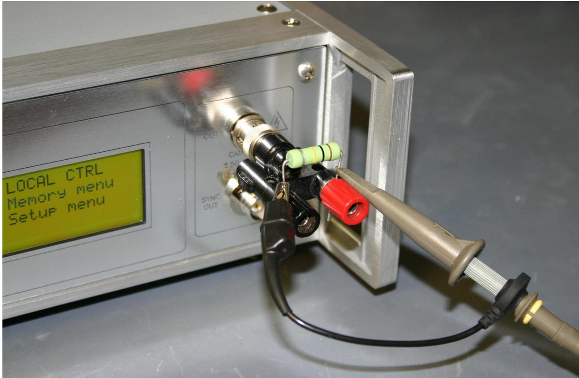
2. Connect a cable from the SYNC connector to the TRIG input of an oscilloscope. Set the oscilloscope to trigger externally.
