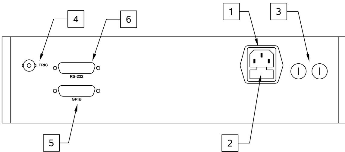
1. AC POWER INPUT. An IEC-320 C14 three-pronged recessed male socket is provided on the back panel for AC power connection to the instrument. One end of the detachable power cord that is supplied with the instrument plugs into this socket.
