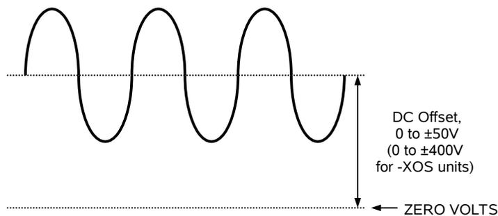
The total output (i.e., the sum of the offset and the amplitude) may not exceed  $\pm 400\text{V}$ .
