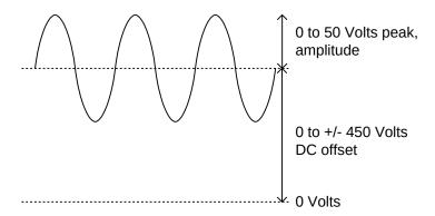
The total output (i.e., the sum of the offset and the amplitude) may not exceed ±500V.
