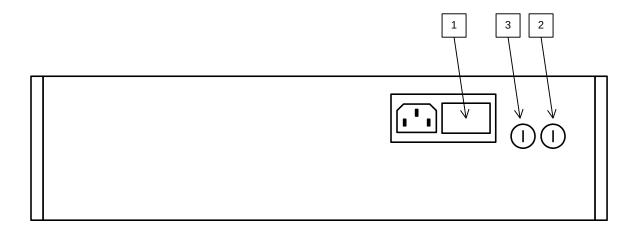
1. <u>AC POWER INPUT</u>. A three-pronged recessed male connector is provided on the back panel for AC power connection to the instrument. Also contained in this assembly is a slow-blow fuse and a removable power selector card that can be removed and repositioned to switch between 110-120V AC in and 220-240V.
