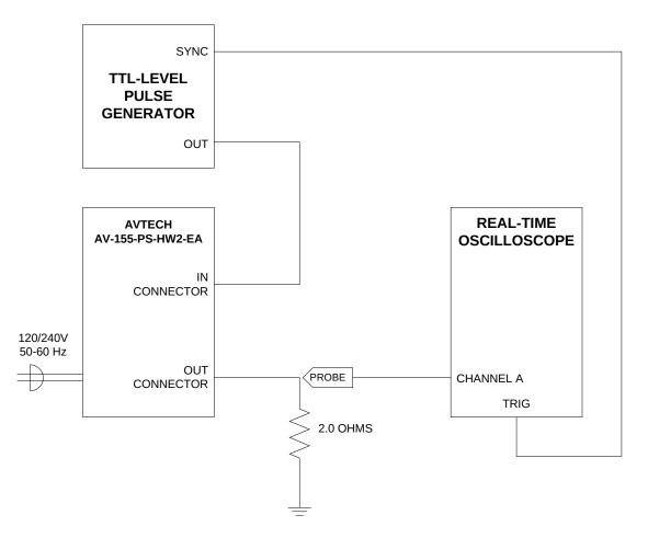
The input and output waveforms for the unit are below. Note that the unit operates as a pulsed constant current source and for that reason the load resistance should be less than 2.5 Ohms (to avoid saturating the output stage) and the load inductance must be exceedingly low (to avoid inductive spikes on the transitions).
