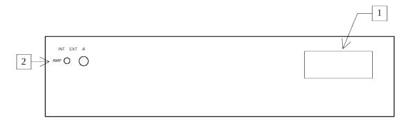
1. <u>AC POWER INPUT</u>. A three-pronged recessed male connector is provided on the back panel for AC power connection to the instrument. Also contained in this assembly is a slow-blow fuse and a removable card that can be removed and repositioned to switch between 120V AC in and 240V AC in.
