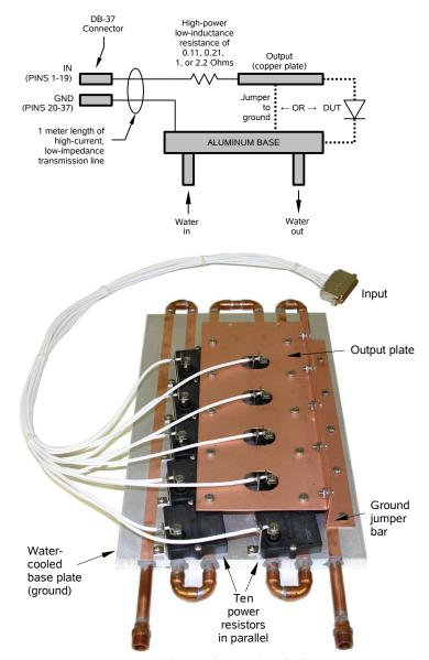
AV-HTL-0R1 (with ground jumper installed)
