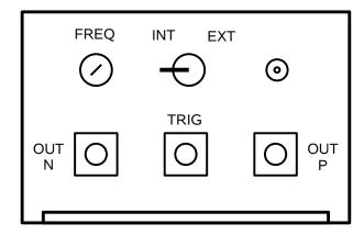
The "OUT N" and "OUT P" SMA connectors are connected to the pulse combiner on the top of the main module, through factory-installed cabling.
