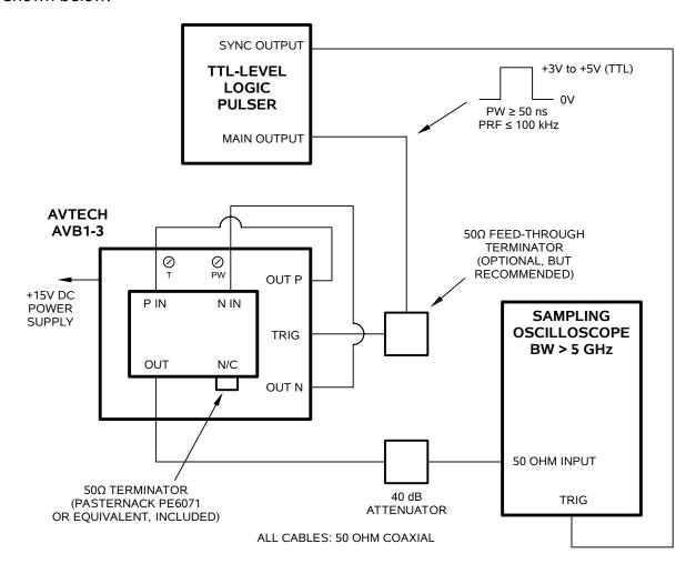
The AVB1-3 generates a positive pulse and a negative pulse internally. These are added together in the pulse combiner located on the top of the main chassis. The OUT P to P IN and OUT N to N IN cables shown in the diagram above are pre-installed on the AVB1-3 (and should never be removed).
