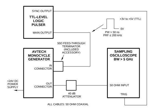
The attenuators are required to prevent damage to the sampling oscilloscope. A 40 dB attenuator with sufficient voltage rating should be used on the main output.
