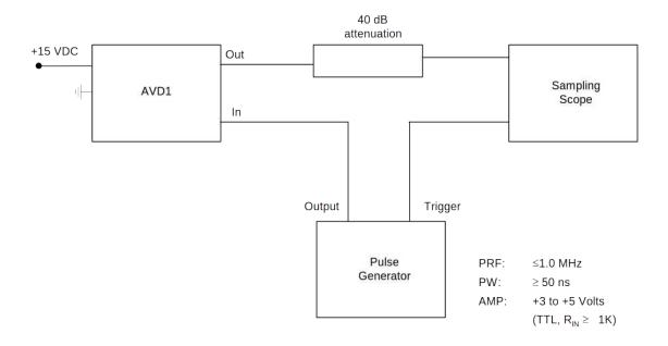
Power line: +15 Volts/0.10 Amps DC, shielded twisted pair, < 3
