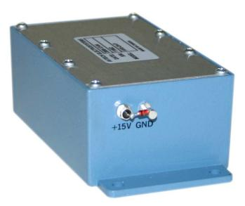
The +15V input terminal is protected with a 1N4746A Zener diode, which will fail as a short if an excessive positive voltage (> 18V), or a negative voltage, is applied to the terminal.
