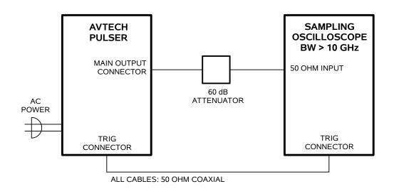
The attenuators are required to prevent damage to the sampling oscilloscope. A 60 dB attenuator (or higher) with an unusually high voltage rating should be used on the main output.
