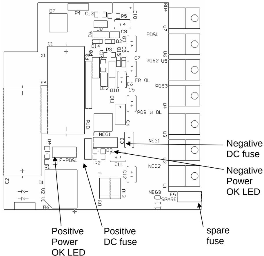
The positive fuse and the spare fuse on this circuit board are 1A slow-blow fuses, Littlefuse part number R452001. (This fuse can be ordered from Digikey, [www.digikey.com](http://www.digikey.com). The Digikey part number is F1343CT-ND). The negative fuse is a 0.5A slow-blow fuse (Littlefuse R452.500, Digikey part number F1341CT-ND).
