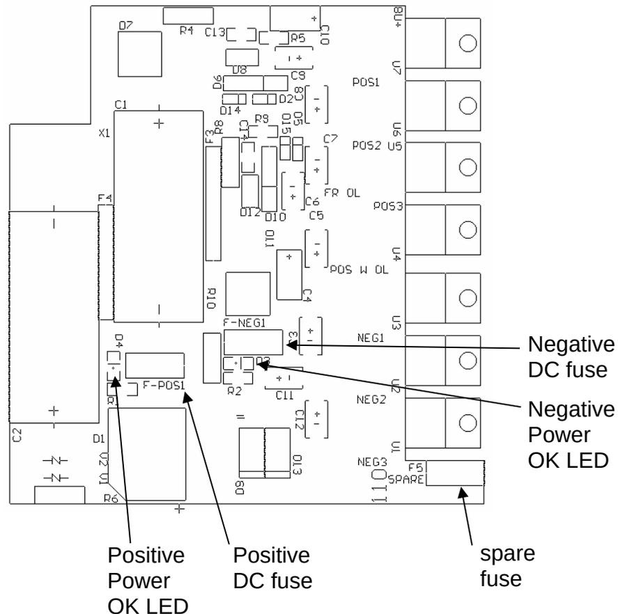
The positive fuse and the spare fuse on this circuit board are 1A slow-blow fuses, Littlefuse part number R452001. (This fuse can be ordered from Digikey, [www.digikey.com](http://www.digikey.com). The Digikey part number is F1343CT-ND). The negative fuse is a 0.5A slow-blow fuse (Littlefuse R452.500, Digikey part number F1341CT-ND).
