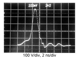
Capacitive loading will inevitably introduce some amplitude loss and transient distortions, as shown below for the example of 20 pF in parallel with 50 Ohms, located at the end of a 24" length of coaxial cable:
