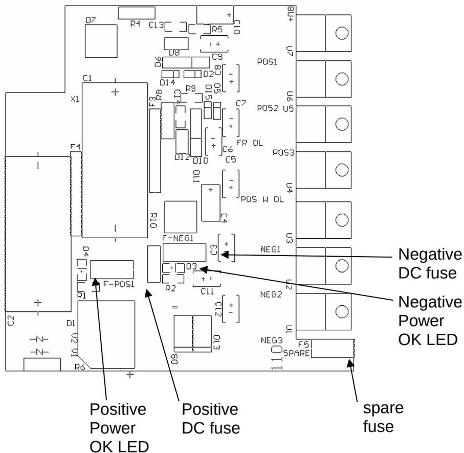
The positive fuse and the spare fuse on this circuit board are 1A slow-blow fuses, Littelfuse part number R452001. (This fuse can be ordered from Digikey, [www.digikey.com](http://www.digikey.com). The Digikey part number is F1343CT-ND). The negative fuse is a 0.5A slow-blow fuse (Littelfuse R452.500, Digikey part number F1341CT-ND).
