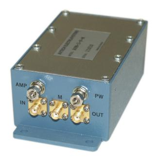
The "AMP" and "PW" controls may be adjusted using a screwdriver. Instruments with the -EA and -EW options will have solder terminal inputs to control the amplitude and pulse width, respectively, instead of screwdriver-adjustable controls. This is shown in
