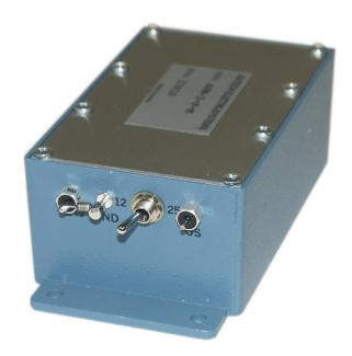
The "12/25" switch should be set in the "12" position if the PRF is less than 12 MHz. For higher PRF the switch should normally be in the "25" position for optimal rise times and pulse widths. Some experimentation may be necessary to find the best operating mode.
