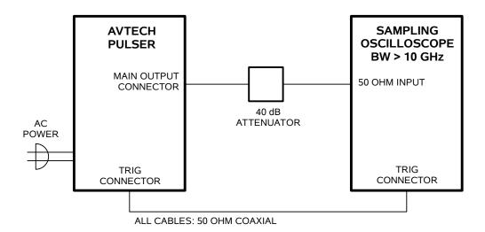
The attenuator is required to prevent damage to the sampling oscilloscope.
