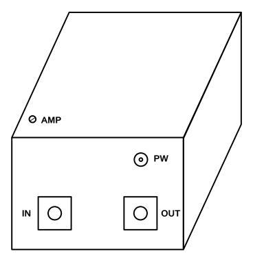
The "AMP" control (a ten-turn trimpot which controls the amplitude) may be adjusted using a screwdriver.
