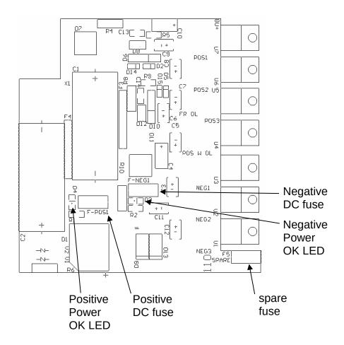
The positive fuse and the spare fuse on this circuit board are 2A slow-blow fuses, Littlefuse part number R452002. (This fuse can be ordered from Digikey, www.digikey.com. The Digikey part number is F1345CT-ND). The negative fuse is a 0.5A slow-blow fuse (Littlefuse R452.500, Digikey part number F1341CT-ND).
