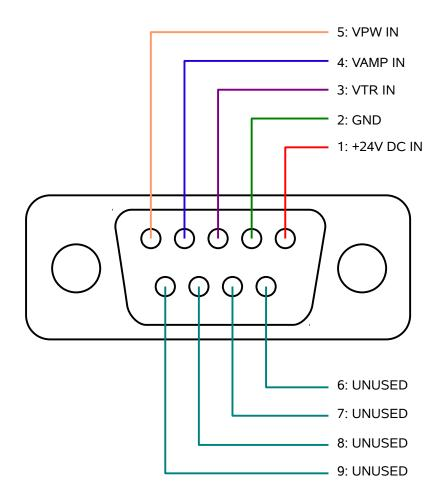
The user-supplied +24V DC power supply must be connected between pins 1 (+24V DC) and 2 (GND).
