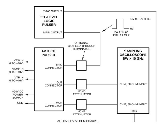
The input impedance of the TRIG connector is 1 k $\Omega$ . This may lead to an impedance mismatch, transmission line reflections, and false triggering. The input impedance can be converted to 50  $\Omega$  simply by adding a feed-through SMA terminator onto the TRIG connector. The Pasternack PE6026 is a suitable terminator (see <a href="http://www.pasternack.com">http://www.pasternack.com</a>).
