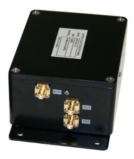
Caution: Voltages as high as ±100V may be present on the center conductor of this output connector. Avoid touching this conductor. Connect to this connector using standard coaxial cable, to ensure that the center conductor is not exposed.
