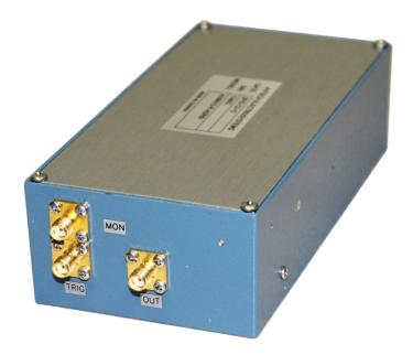
Caution: Voltages as high as ±100V may be present on the center conductor of this output connector. Avoid touching this conductor. Connect to this connector using standard coaxial cable, to ensure that the center conductor is not exposed.
