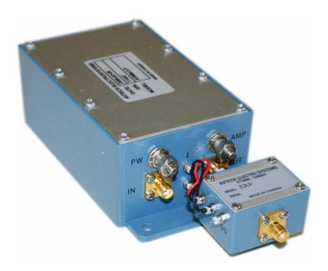
The "AMP" and "PW" controls may be adjusted using a screwdriver.
