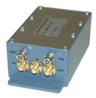
The "AMP" and "PW" controls may be adjusted using a screwdriver. Units with the -EA or -EW options will have solder terminals instead of screwdriver-adjustable controls.
