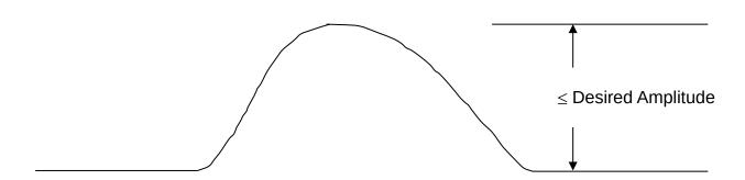
Having obtained a display of the form shown above, the desired pulse width is then obtained by adjusting the two front panel pots TR and TF. Rotate TR counter clockwise from the positive set in step 2) until a sharp 100 ps leading edge is observed. Then rotate TF counterclockwise until the desired pulse width and fall time are obtained.
