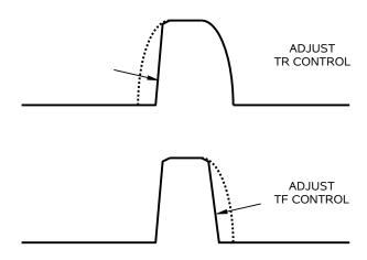
Further iterative adjustments of TR and TF will be necessary to simultaneously obtain the lowest rise time, lowest fall time, the desired pulse width, and pulse top shape, and low spurious signal level. In addition some additional adjustment of signal level may be necessary to obtain the desired amplitude. If the input frequency is then changed it will be necessary to readjust AMP, TR and TF to establish the required pulse shape.
