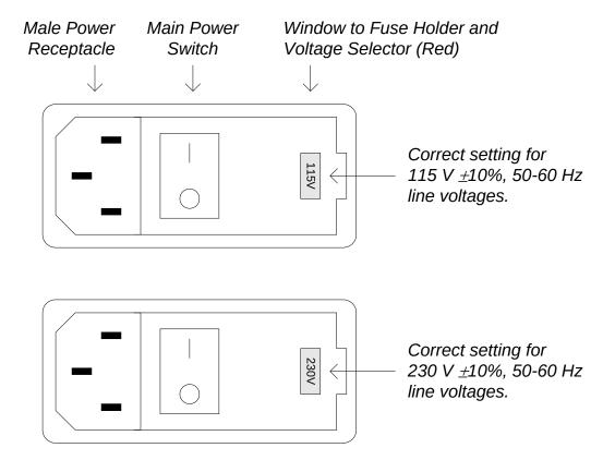
If the voltage selector is not set for to proper voltage, use a small flat-head screwdriver to pry open the voltage selector panel, as shown below:
