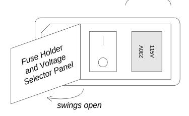
Once the panel is open, the red fuse holder / voltage selector should be visible. To change the voltage setting, pull out the red fuse holder / voltage selector and rotate it so that the proper voltage marking will shown through the panel window. Re-install the red fuse holder / voltage selector, and close the panel.
