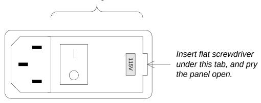
Fuse Holder and Voltage Selector. After opening the panel, the red plastic fuse holder and voltage selector will be visible.
