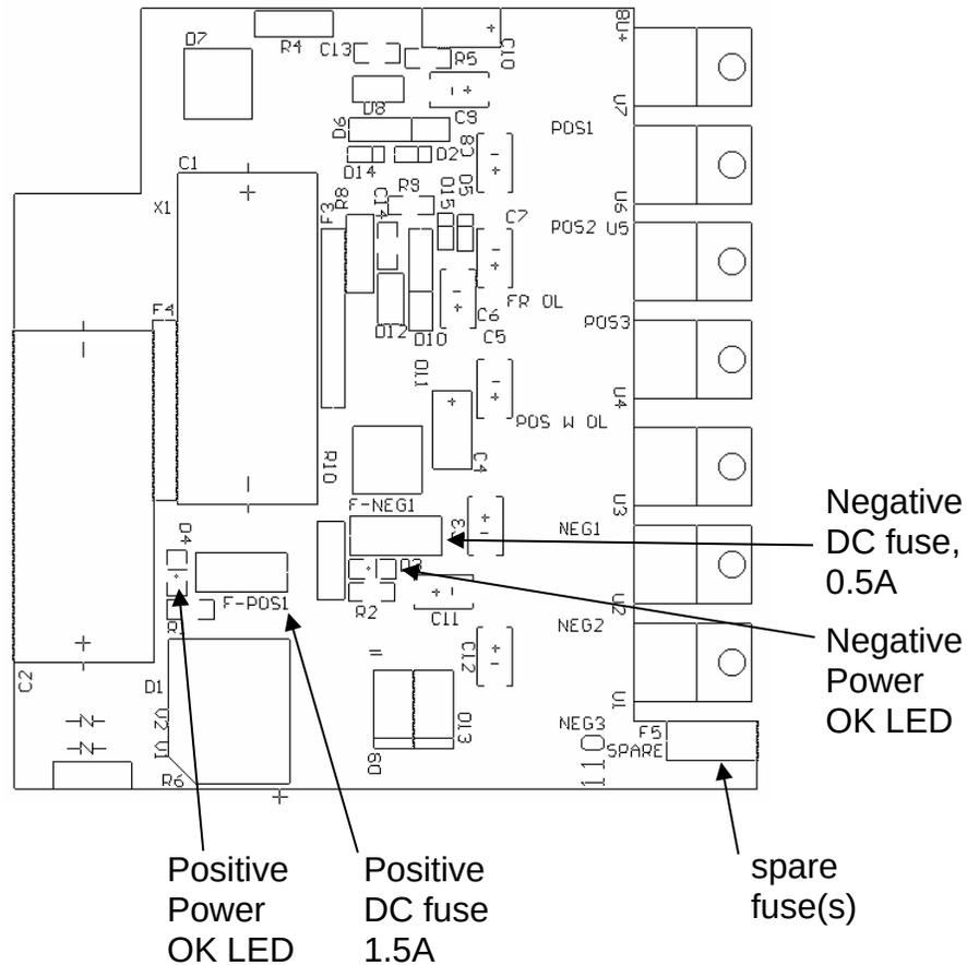
The positive fuse and the one of the spare fuses on this circuit board are 1.5A slow-blow fuses, Littelfuse part number R45201.5. (This fuse can be ordered from Digikey, [www.digikey.com](http://www.digikey.com). The Digikey part number is F1344CT-ND).
