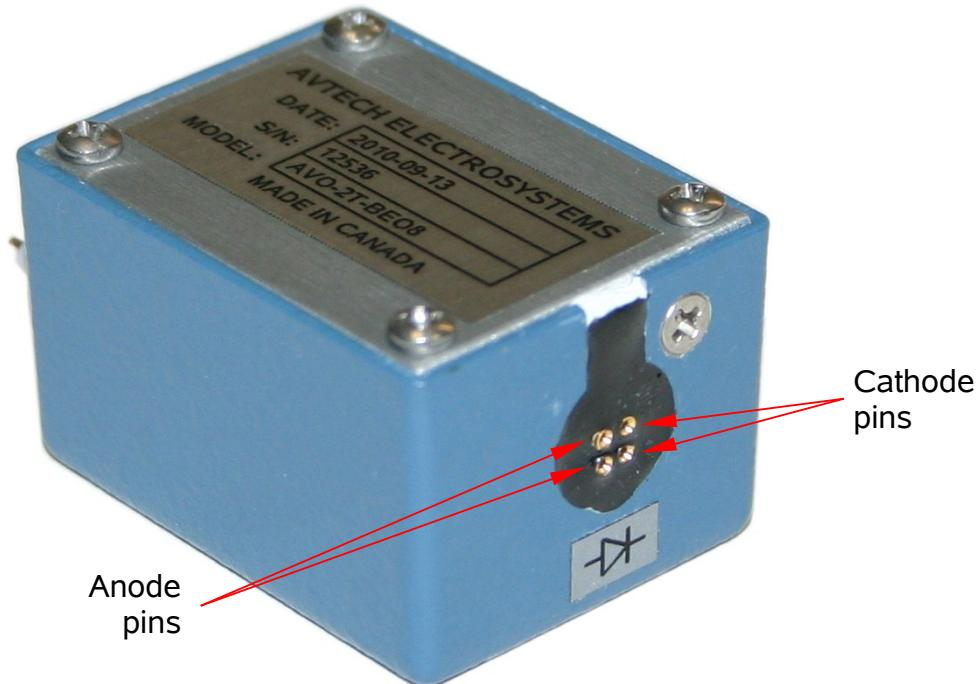
Four pin sockets are provided. The two on the left are shorted together, and one or both must connect to the device anode.
