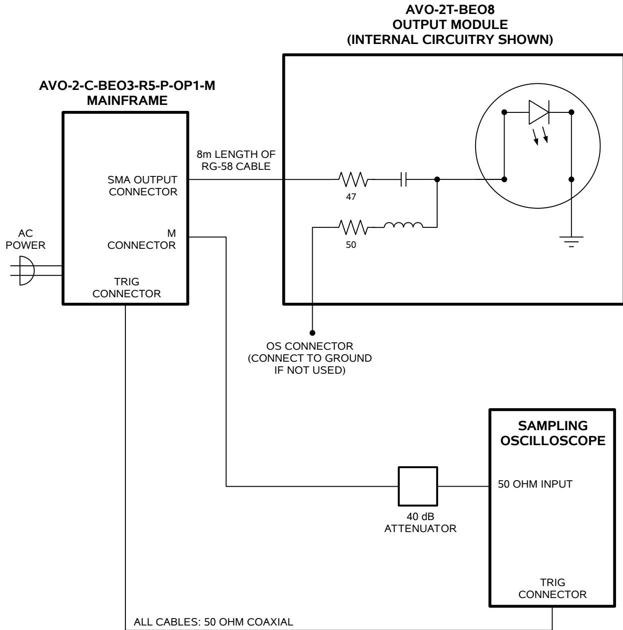
When used with the AVO-2-C-BEO3-R5-P-OP1-M, pulses of up to +2A and widths of 17 ns may be obtained.
