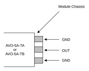
The diode load and series current limiting resistor should be connected between the OUT and GND terminals using very short leads (<0.5 cm). The series current limiting resistors must be non inductive. Carbon composition resistors are suitable for this application. The voltage across the resistor-diode load may be monitored by means of a high impedance scope probe.
