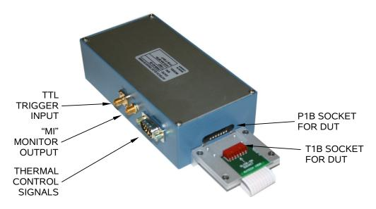
The externally-generated TTL trigger signal must be applied to the SMA connector shown above. The input impedance is 50 Ohms.
