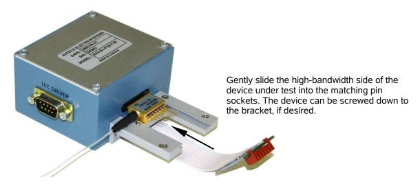
If present, the T1B slide-on socket assembly can then be slid onto pins 1-7, as shown below:
