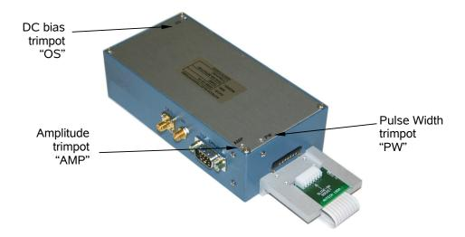
Rotating a trimpot clockwise will increase the controlled parameter (amplitude, pulse width, or DC bias current).
