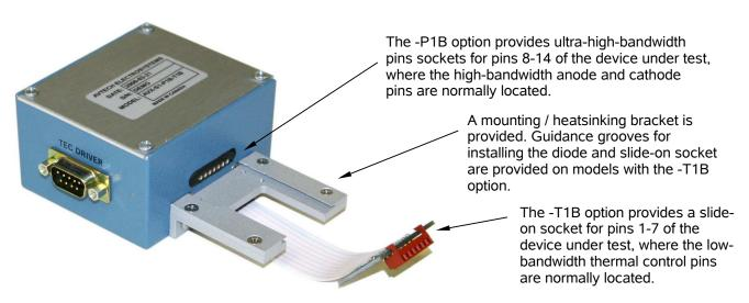
The diode is first installed by sliding pins 8-14 into the "P1B" pin sockets, as shown below:
