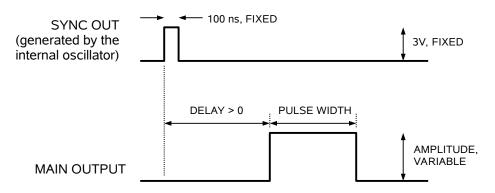
If the delay is negative, the order of the SYNC and OUT pulses is reversed:
