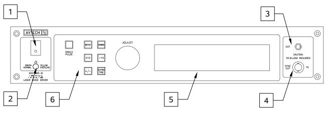
1. <u>POWER Switch</u>. This is the main power switch. When turning the instrument on, there is normally a delay of 10 seconds before anything is shown on the main display, as the internal operating system boots up.
