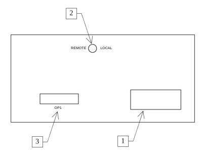
(1) <u>FUSED CONNECTOR</u>, <u>VOLTAGE SELECTOR</u>. The detachable power cord is connected at this point. In addition, the removable cord is adjusted to select the desired input operating voltage. The unit also contains the main power fuse.
