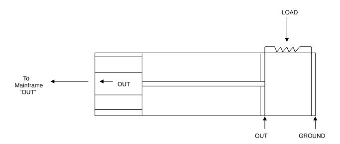
Note that the load should be greater than 1.0 Ohms (10 Watts).
