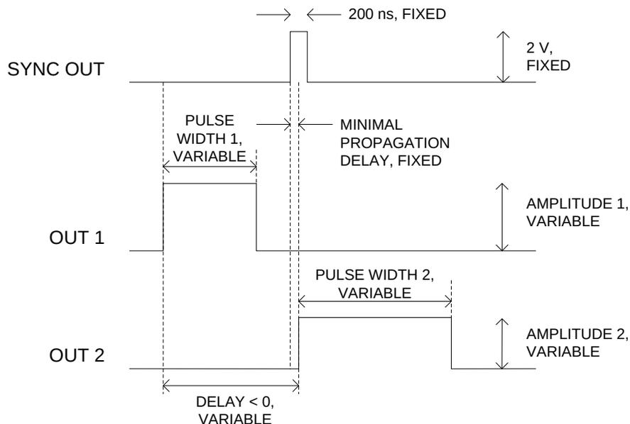
*Basic Output Pulses for Delay < 0*
