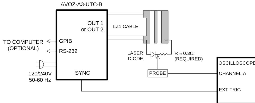
The equipment should be connected in the general fashion shown above. Since the AVOZ unit provides an output pulse rise time as low as 30 ns a fast oscilloscope (at least 100 MHz) should be used to display the waveform.
