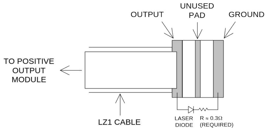
In the above diagram, the diode is oriented for positive current flow. Reverse the diode for negative operation.
