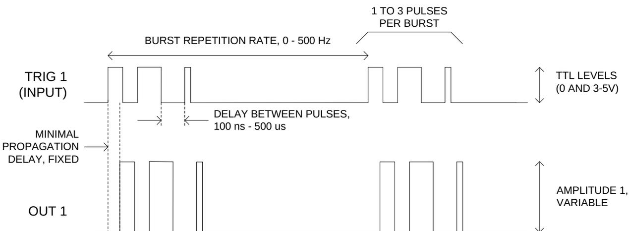
The Channel 2 timing is similar, except that the “DELAY BETWEEN PULSES” can vary from 30 ns to 500 us.
