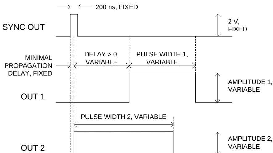
*Basic Output Pulses for Delay > 0*
