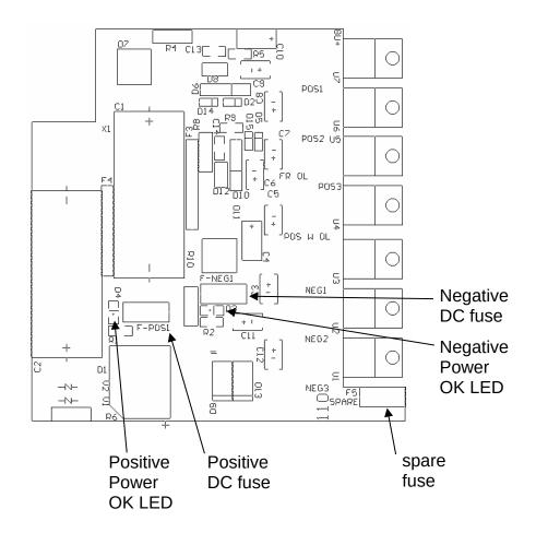
The positive fuse and the spare fuse on this circuit board are 1A slow-blow fuses, Littlefuse part number R452001. (This fuse can be ordered from Digikey, <a href="https://www.digikey.com">www.digikey.com</a>. The Digikey part number is F1343CT-ND). The negative fuse is a 0.5A slow-blow fuse (Littlefuse R452.500, Digikey part number F1341CT-ND).
