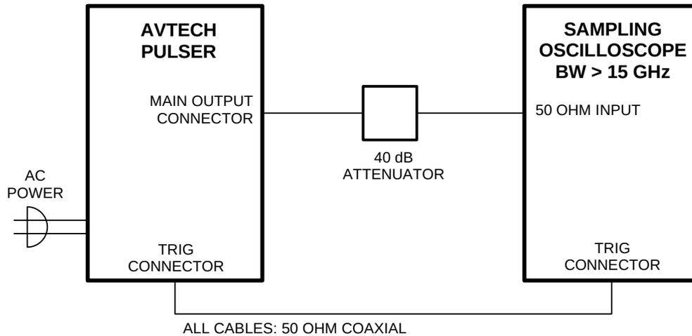
The attenuators are required to prevent damage to the sampling oscilloscope. A 40 dB attenuator with sufficient voltage rating should be used on the main output. Factory tests are conducted using Mini-Circuits model BW-S20W2+ attenuators.
