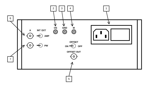
1. <u>AC POWER INPUT</u>. A three-pronged recessed male connector is provided on the back panel for AC power connection to the instrument. Also contained in this assembly is a slow-blow fuse and a removable card that can be removed and repositioned to switch between 120V AC in and 240V AC in.
