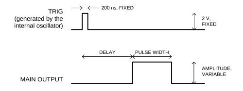
When triggered externally, the TRIG connector acts as an input. The delay controls do not function in this mode. This illustrated below:
